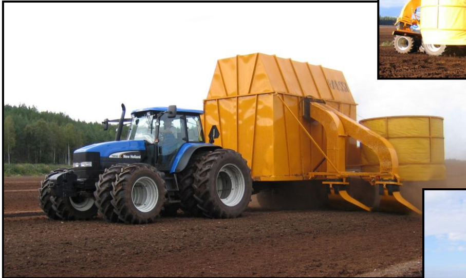
HIK-340 equipped with dustcyclon PSL-300
